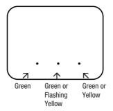
If the Middle light is not on, then the device does not have a valid connection to our Web Servers. Try the following.
